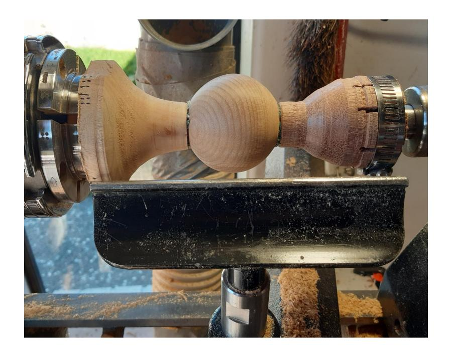
Cut off sphere and position between home-made jigs
