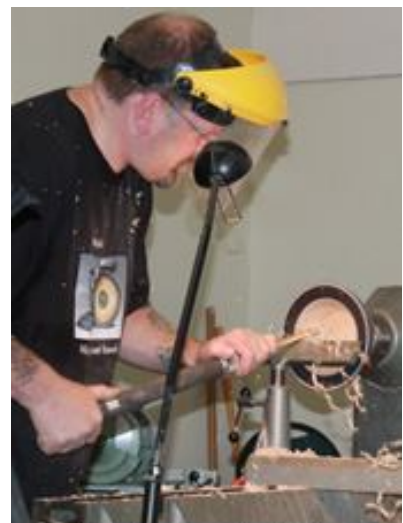
Finishing cut on the inside
